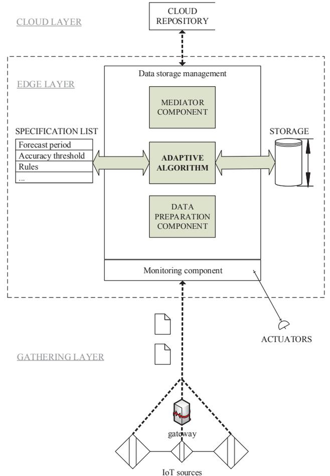
Fig. 1. Architecture for Edge storage management
