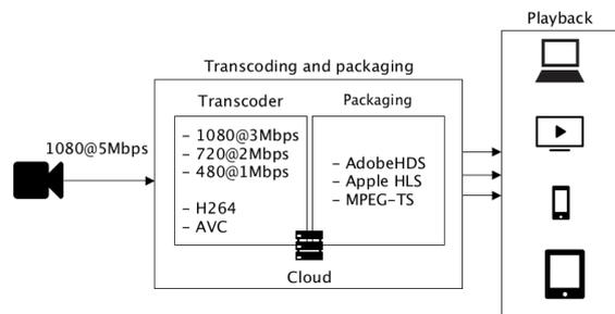
Figure 3: Cloud based solution for live streaming services
