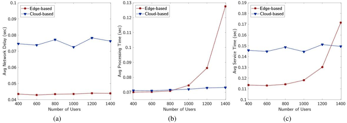
Figure 7: Comparison of the average network delay (a) average processing time (b) and average service time (c) in the edge scenario using a cloud scheduler and the edge scheduler we developed.
